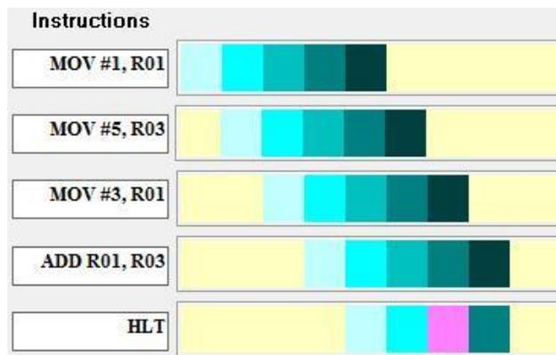
Figure 6. Pipeline with no bubbles.
